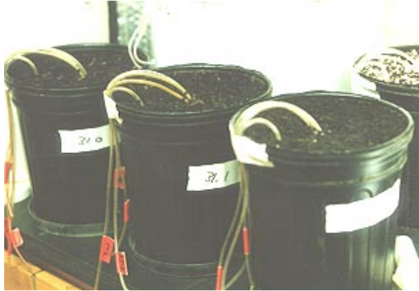
Figure 1. Tubes inserted into pots at varying depths, used to measure oxygen levels before and during growth of plants.
