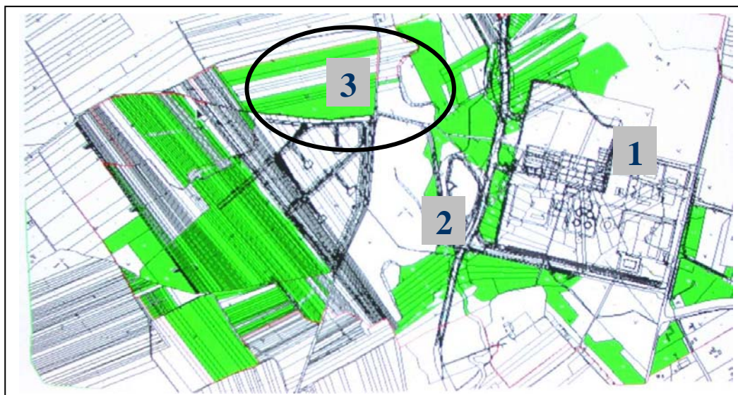
Figure 2: Location Localization of willow plantation (authors: The City of Lodz Office): 1 – The main building of Water Treatment Plant; 2 – The sludge lagoon; 3 – The experimental willow plantation.
