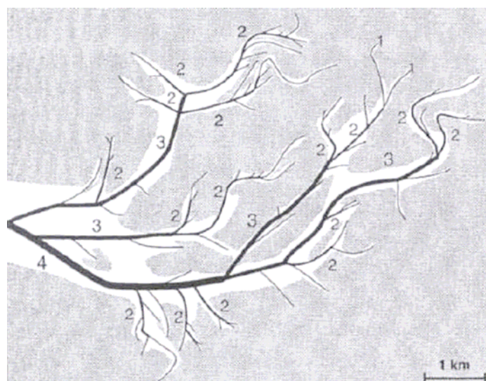
Figure 2.2 Branching channel pattern. The smallest channels are assigned to the first order. Two first order channels merge into a second order channel and so on (from Cleveringa and Oost, 1999).
