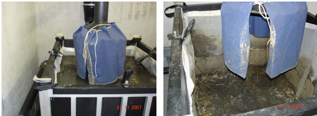
Figure 7. Operation of compost filters with different structure material – left figure bark, right figure straw.
