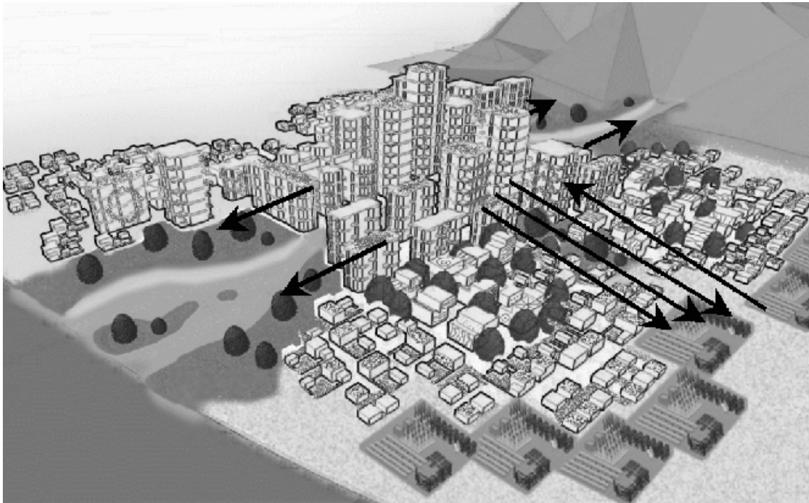
Figure 2: Idealised flow scheme from a complex citywide ecosan system. In the less densely settled areas outside of the city centre, flow streams can be collected decentrally and used locally in gardens or urban agriculture. For the more densely settled city centre, urine, faeces and greywater may have to be collected using (semi-) centralised systems and used to irrigate green areas or for food production outside the city limits (source: GTZ)
