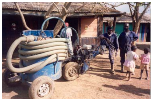
Faecal sludge emptying machine- VacuTug Nairobi - Photo: Jo Smet IRC
